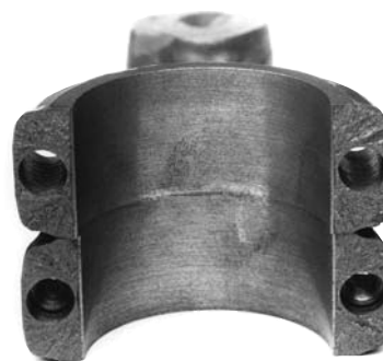
Figure 7 Fracture Split Connecting Rod in C70S6 Air Cooled Grade
