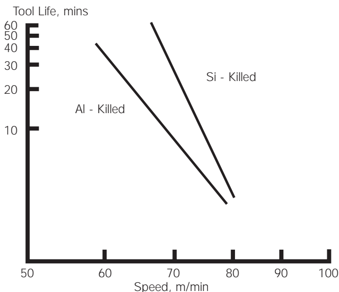
Figure 5 Comparative Machinability of 080A47 Grade with and without an Aluminium Addition
