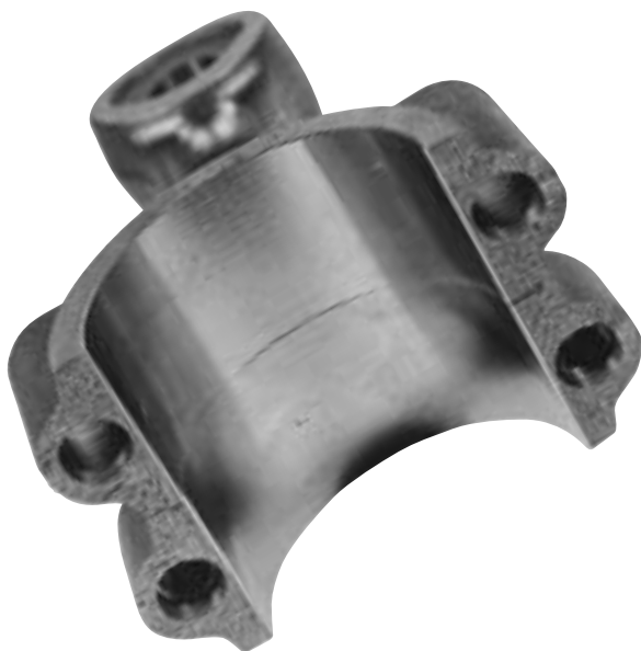
Figure 7 Fracture split connecting rod in C70S6 air cooled grade
