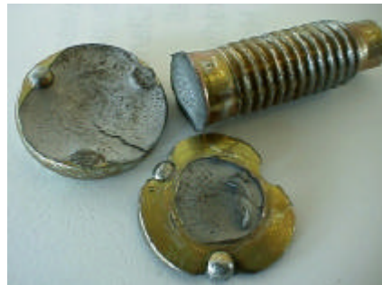
Figure 7. Example of brittle fracture caused by hydrogen pick-up during plating.
