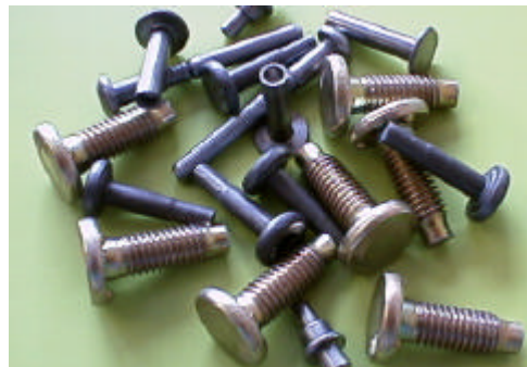
Figure 5. Typical cold headed components produced from >800MPa Dupla wire.
